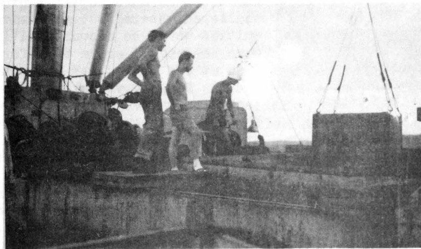
FIG. 5 - A PAIR OF THE SHIP'S WINCHES BEING USED TO LOWER A FISH BOX TO THE UPPER DECK.
