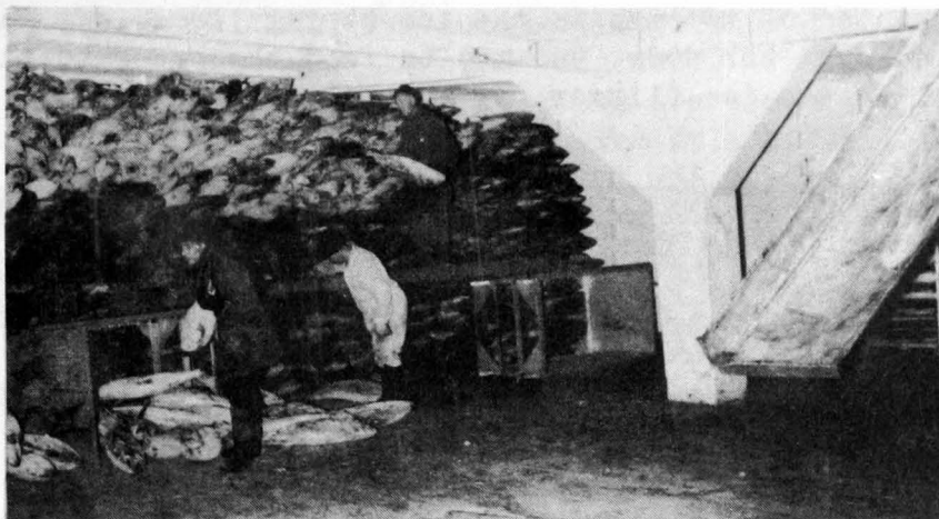
FIG. 12 - STACKING FROZEN TUNA IN A STORAGE HOLD. NOTE THE METAL CHUTE FOR GUIDING THE TUNA.
